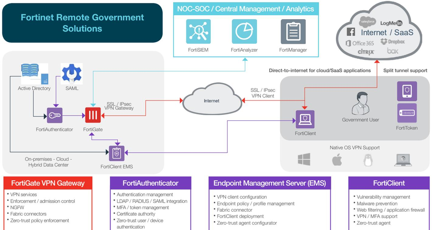
Figure 1: Fortinet solution deployment for standard government worker.
